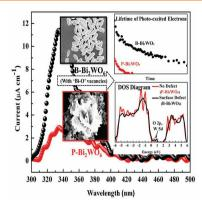
Bi<sub>2</sub>WO<sub>6</sub> nanobipyramid is successfully fabricated via a facile strategy in which "Bi-O" vacancy pairs are key to increase its solar-light photoactivity.
