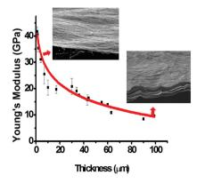
The mechanical properties of graphene oxide (GO) papers are shown to be thickness-dependent. This dependence arises from the micro- and macrostructure formed during the fabrication process; microscopy studies reveal that corrugations, void defects, and surface wrinkles all influence the mechanical properties. Establishing this structure-property relationship is expected to enable improved guidelines for the application of GO to mechanical structures.
