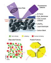
A nanoscale liquid imaging platform is developed to track lithium intercalation in LiFePO<sub>4</sub> electrodes. The results show that the intercalation pathway strongly depends on the particle morphology and synthesis protocol. Highly faceted ellipsoidal particles intercalate sequentially, with a small number of actively intercalating particles and low electrode utilization. Platelet particles, on the other hand, intercalate simultaneously with a more uniform current distribution.
