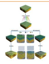
By taking advantage of the dual metal substrate of Ni-coated Cu foils, the precise control of layer number of graphene by ion implantation is demonstrated and the layer number of graphene strictly corresponds to the implantation fluence as expected. Besides, the formation mechanism is explored by the experimental analysis in detail and confirmed by the theoretical calculations.
